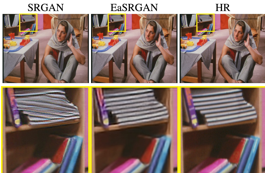
Fig. 1: Unlike the 4\times upscaling in SRGAN (left), our EaSRGAN output (center) suppresses artifacts to obtain a result close to the original HR image (right). The bottom row shows the zoomed-in yellow box.
