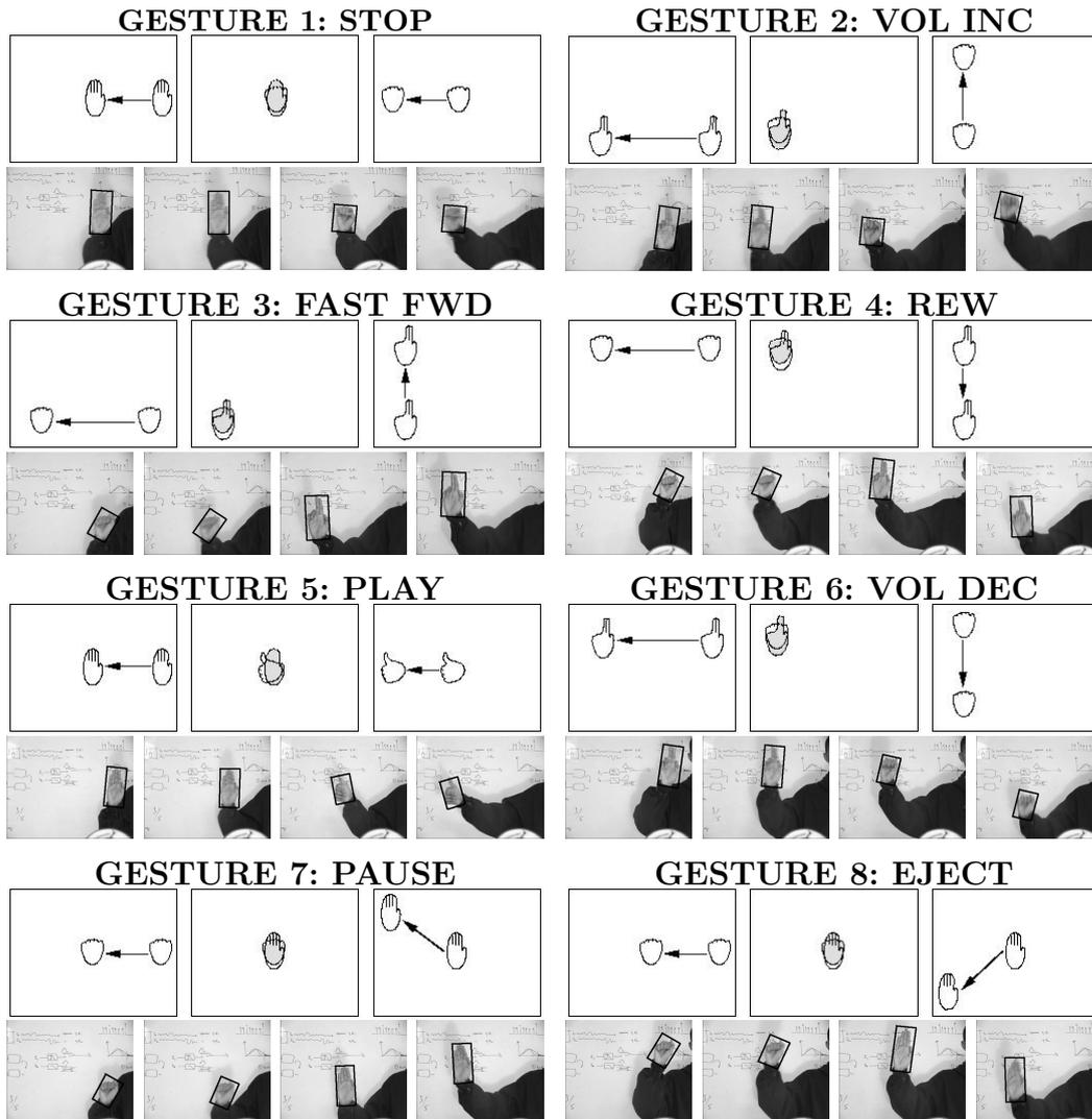
Fig. 2. A sample gesture set for controlling an audio player such as Winamp<sup>©</sup>: the gestures cannot be distinguished on the basis of shape or trajectory alone. The top row for each gives a schematic, the bottom one shows representative tracker output frames. Colour MPEG videos at <http://www.ee.iitb.ac.in/~sumantra/pr105a/> clearly show the non-uniform background and shadows.
