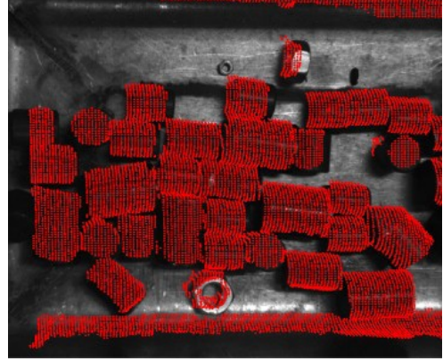
Fig. 2. Projection of laser data on image, similar to [39]
