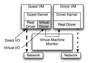
Figure 1: I/O paths in a virtual machine.
