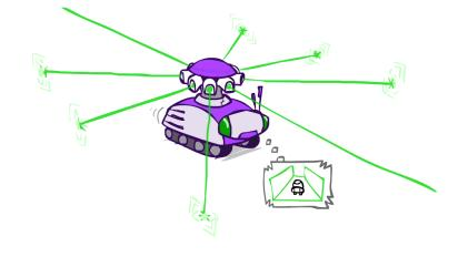
Sensor model: can read in which directions there is a wall, never more than 1 mistake Motion model: may not execute action with small prob.
