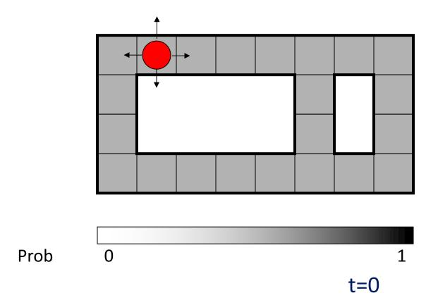
Robot can take actions N, S, E, W Detects walls from its sensors
