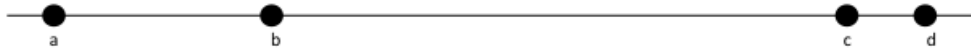
Figure 1.1: A simple one dimensional example for showing that Lloyd's algorithm may not give any approximation guarantees. Consider four points as shown above and let their labels also be their x coordinates. For k = 3 , the optimal centers are located at a, b , and (c + d)/2 with cost (d - c)^2/2 . However, if the Lloyd's algorithm picks a, c, d as the initial 3 centers, then the algorithm outputs centers (a + b)/2, c, d with cost (b - a)^2/2 which may be arbitrarily bad compared to the optimal.
