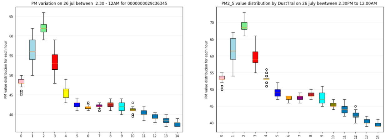
Fig. 1. Low Cost sensor's PM 2.5 values on the left vs. a co-located TSI DustTrak's PM 2.5 values on the right, on a sample day. While their costs are 30 USD and 10K USD respectively, i.e. an order of magnitude different, their measured PM values are almost identical.
