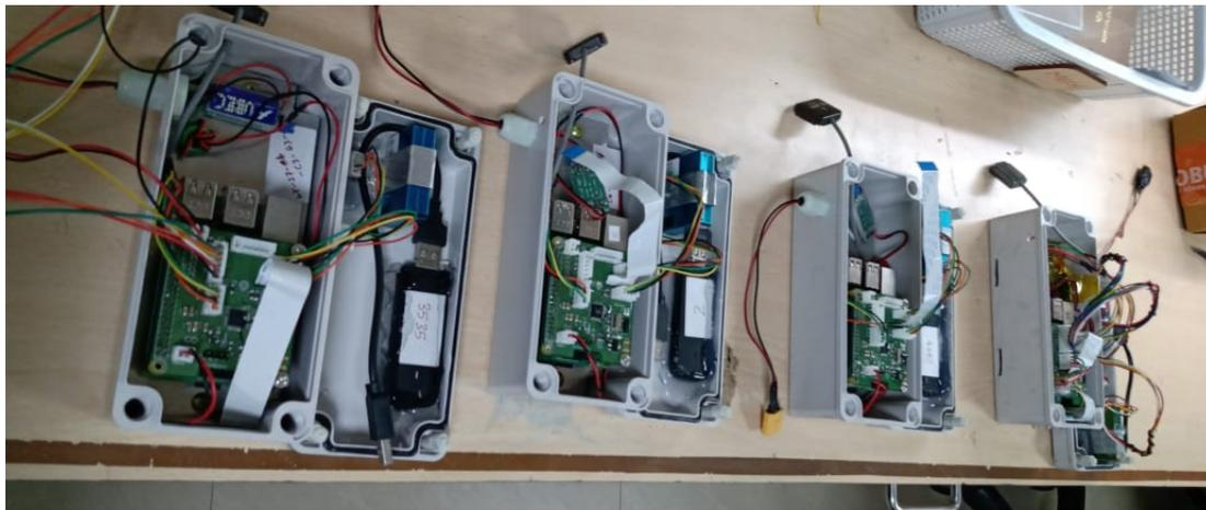
Fig. 3. Hardware platform second prototype showing the sensors, micro-controller, our custom PCB etc., inside ABS plastic boxes.
