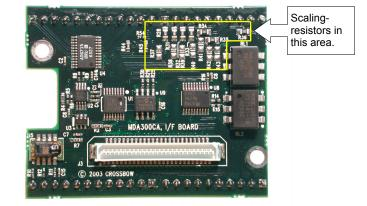
Figure 6-3. Photo of backside of the MDA300CA.
