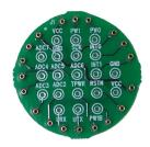
Figure 7-1. Photo of top-side of an MDA500CA for the MICA2DOT.
