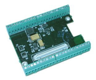
Figure 6-1. Top view of an MDA300CA. This is the side a MICA2 mote would be attached.
