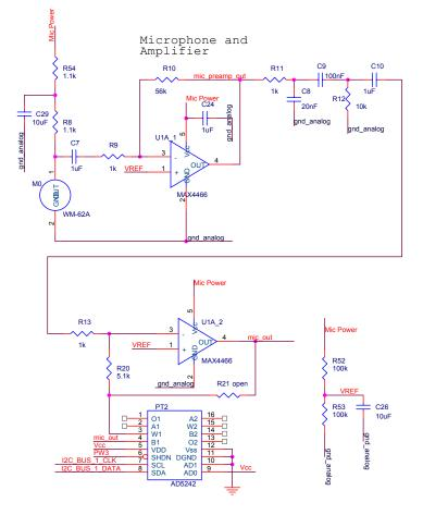
Figure 3-5. MTS310CA Schematic of Microphone and Amplifier.
