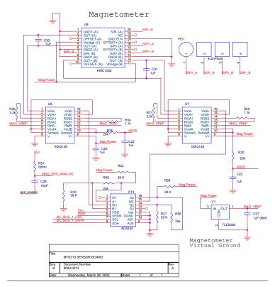
Figure 3-4. MTS310 Schematic of Magnetometer.
