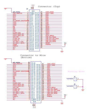
Figure 3-2. MTS310CA Schematic of 51-pin Connector Pin-outs
