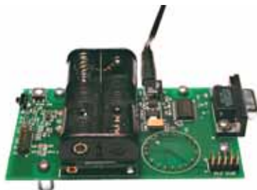
Figure 4-1. MICAz/MICA2 plugged into top-side of an MIB510. Figure 4-2. MICA2DOT plugged into bottom-side of an MIB510.
