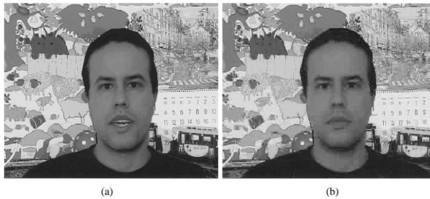
Fig. 12. Example frame from a video sequence rendered from (a) a 3-D head model and watermarked animation parameters and (b) a similar frame after subsequent MPEG-2 video compression at 600 kbit/s.
