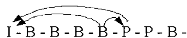
Fig. 10. Example for the structure of I, P, and B frames in a GOP.
