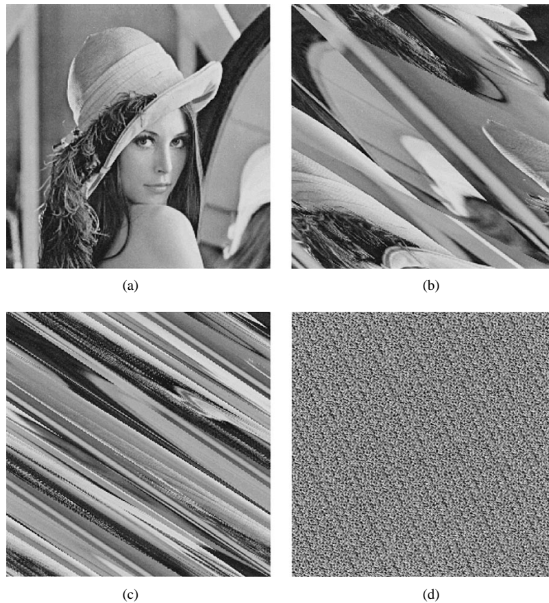
Fig. 6. Example automorphism with the “cat map.” (a) is the original image. (b)–(d) show the automorphism of (a) after one, two, and ten iterations, respectively.
