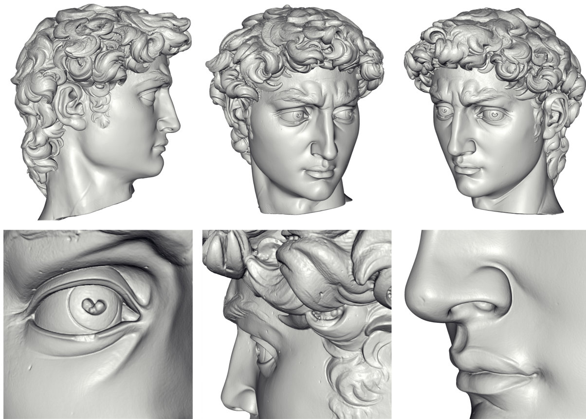
Figure 8: Several images of the reconstruction of the head of Michelangelo's David, obtained running our algorithm with a maximum tree depth of 11. The ability to reconstruct the head at such a high resolution allows us to make out the fine features in the model such as the inset iris, the drill marks in the hair, the chip on the eyelid, and the creases around the nose and mouth.
