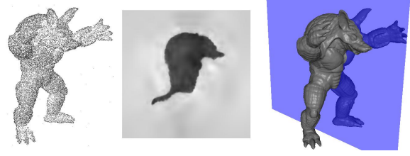
Figure 2: Points from scans of the “Armadillo Man” model (left), our Poisson surface reconstruction (right), and a visualization of the indicator function (middle) along a plane through the 3D volume.
