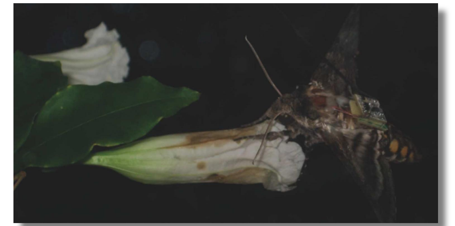
Untethered moth with RFID measurement sensor (< 1 cm 2 , weighs 0.25 g)
