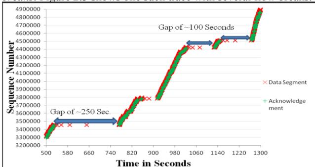
Figure 2.3: Long flow breaks in Airtel GPRS connection in downlink direction.
