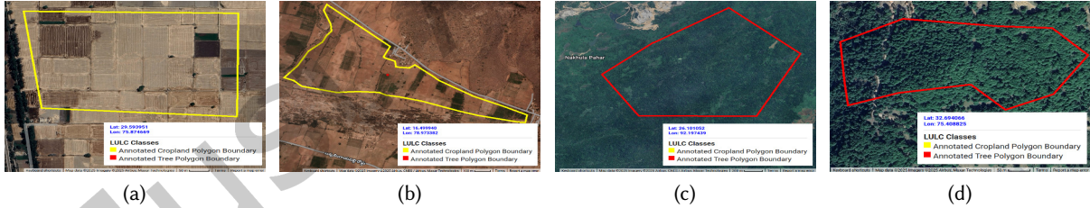
Fig. (3) Visual examples of cropland & tree annotations: Subfigures (a,b) illustrate polygons covering croplands, while (c,d) show tree-covered polygons.
