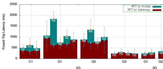
Figure 4: RTT to the measurement server and cellular gateways
