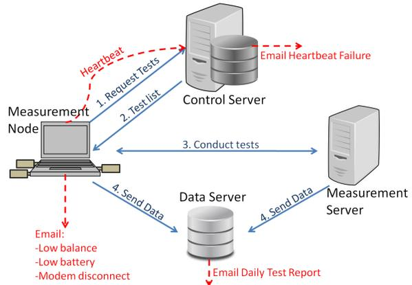
**Figure 1: Measurement architecture. Solid lines test execution steps. Dashed lines show suite health monitoring components**
