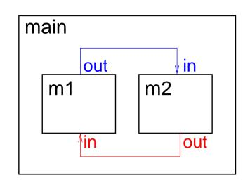
Formal parameters (in) are substituted with the actual parameters (m2.out, m1.out) when the module is instantiated.
