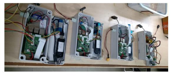
Fig. 3. Hardware platform second prototype showing the sensors, micro-controller, our custom PCB etc., inside ABS plastic boxes.
