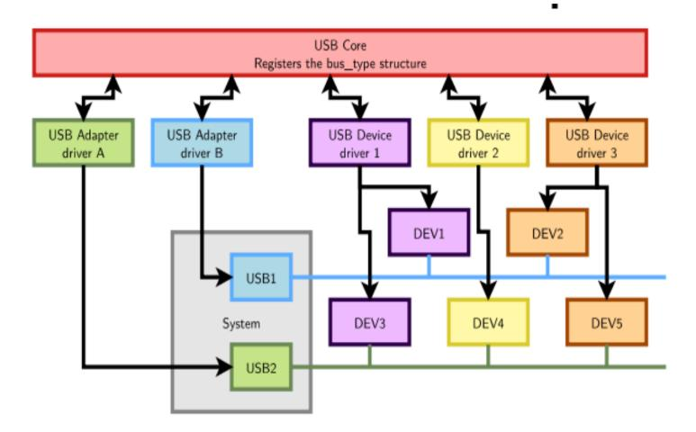
A single driver for compatible devices, though connected to buses with different controllers.
