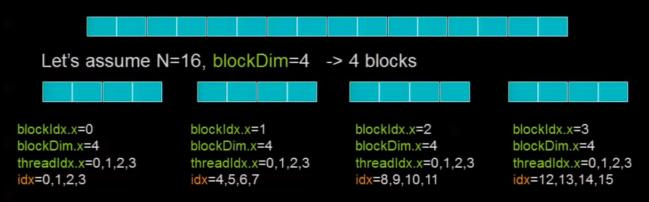
int idx = blockDim.x \* blockId.x + threadIdx.x; will map from local index threadIdx to global index NB: blockDim should be >= 32 in real code, this is just an example
