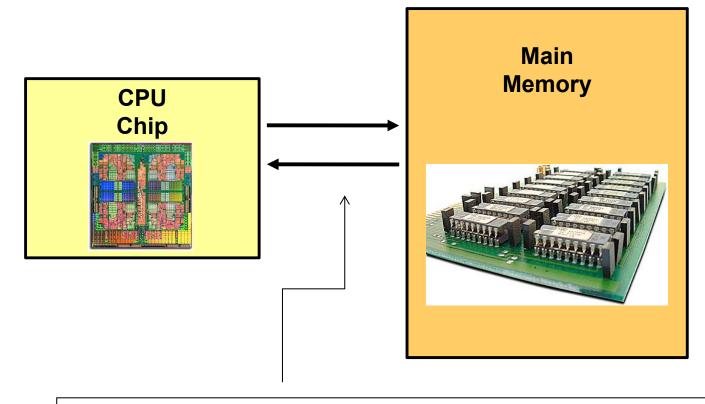
This path is relatively slow, forcing the CPU to wait for up to 200 clock cycles just to do a store to, or a load from, memory.
