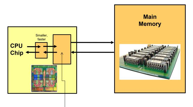
The solution is to add intermediate memory systems. The one closest to the CPU is small and fast. The memory systems get slower and larger as they get farther away from the CPU.
