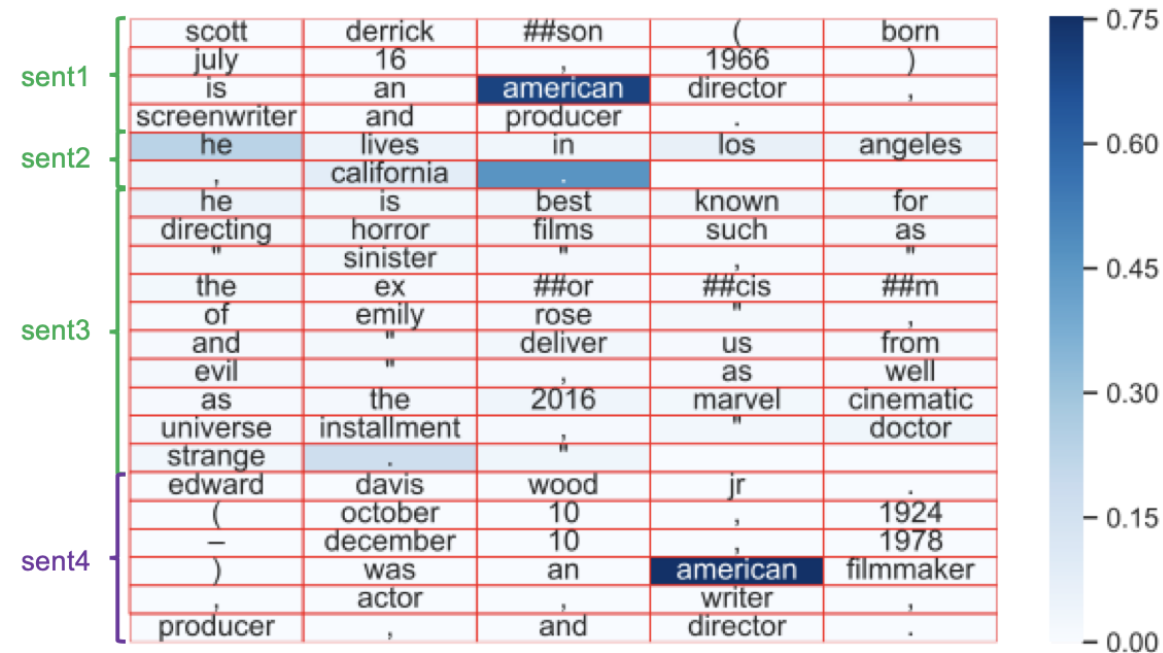
Figure 5: Attention heatmap of a sample from dev set. Each cell is a word piece token returned by BERT. Sentences with different colors are from different documents.
