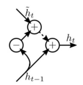
In a variation on the dropout philosophy, Krueger et al. (2017) proposed Zoneout where "instead of setting some units' activations to 0 as in dropout, zoneout randomly replaces some units' activations with their activations from the previous timestep." this "makes it easier for the network to preserve information from previous timesteps going forward, and facilitates, rather than hinders, the flow of gradient information going backward"
