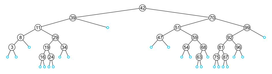
The values which may be inserted at any empty node depend on the surrounding nodes
