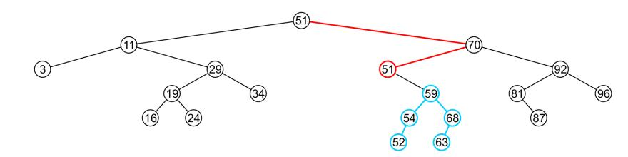
We delete the node containing 51 and assign the member variable left\_tree of 70 to point to 59
