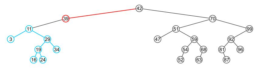
The node containing 39 is deleted and left\_node of 42 is updated to point to 11 – Notice that order is still maintained
