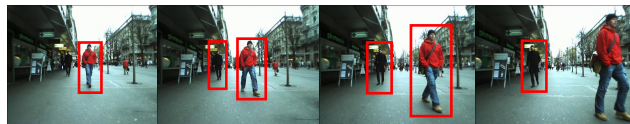
(b) A fast running detector with lower accuracy is able to run detections on all frames but unable to detect all pedestrians in the frame. Nevertheless, it may still outperform a slower detector.
