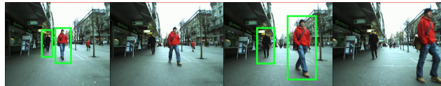
(a) A slower running detector which has a higher accuracy has to skip frames in order to maintain real-time operation. When too many frames have to be skipped to keep up with the real-time performance, a lot of pedestrians go undetected resulting in a poor performance on the application level.
