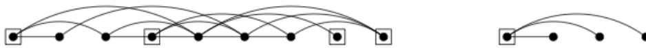
Figure 2.4: Two graphs with a vertex order and the result of the greedy algorithm for Independent Set.
